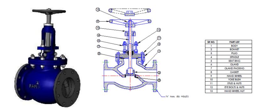
**SDNR/SDSL** – This has an opening that forms a seat onto which a movable plug, called disk or disc, which canbe screwed in to close (or shut), or screwed out to open the **valve**. **Valves** offers two varieties of Globe **Valves**: **SDNR**, **Screw Down Non-Return**; and SDSL, Screw Down Screw Lift.
