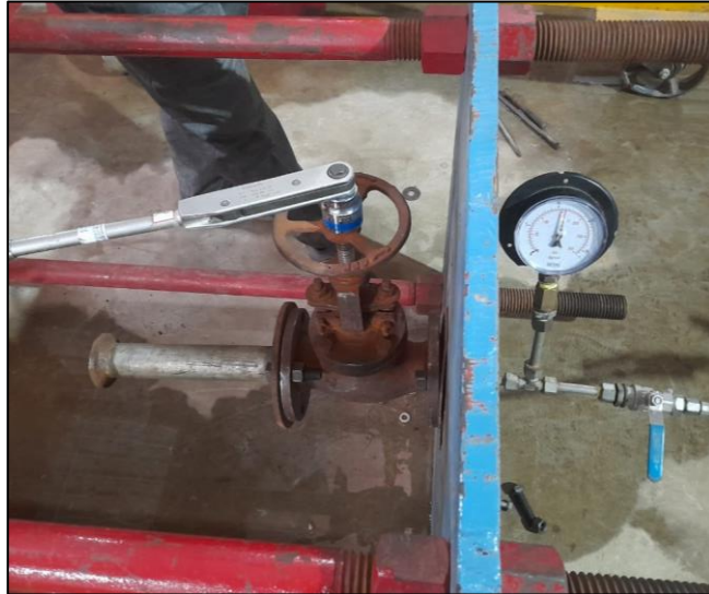
Figure 1: 50NB PN16 TORQUE TEST SETUP
