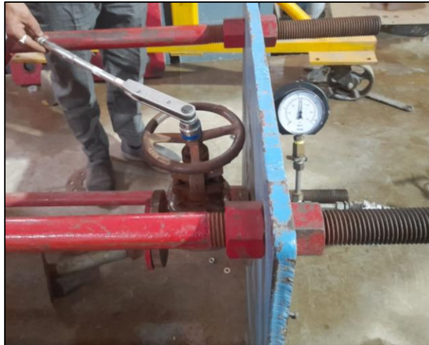
Figure 1: 40NB PN10 TORQUE TEST SETUP
