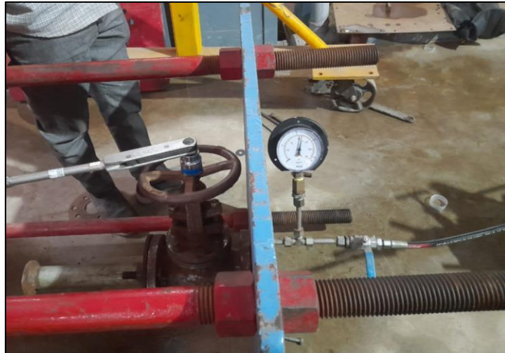
Figure 1: 65NB PN10 TORQUE TEST SETUP
