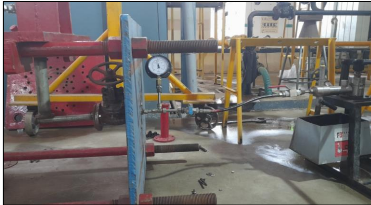
Figure 1: 40NB PN10 PIPE WRACKING SETUP
