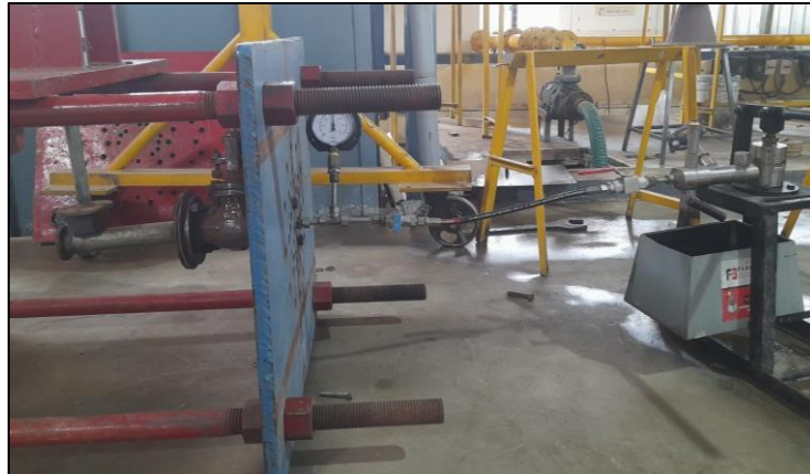
Figure 1: 50NB PN16 PIPE WRACKING SETUP
